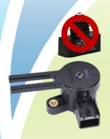
TIG31066 rotary switch for hydraulic brakes (when brake pedal position message is not broadcast by the CANBus) – must be used with TRCM control module – previously plunger type switch which is no longer available was used with ABS interface or speed switch
