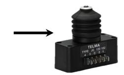
The Telma rotary type switch replaced the plunger type switch and is the current switch if needed. It sends a variable increasing voltage to the TRCM as the brake pedal is applied.
