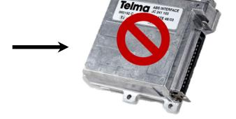
The Telma speed switch was used to connect to the vehicle speed signal using a hard wired connection to provide low speed cutoff for vehicles that were not equipped with ABS
